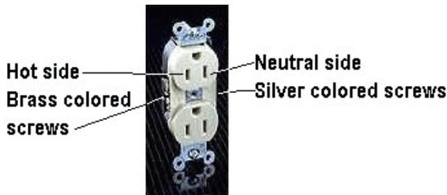
How do you correct this if your polarity is reversed? Turn the power off to the outlet by opening the breaker or pulling the fuse. Check the outlet again to be sure it is dead. Remove the outlet, the hot wire, (should be the black wire) probably is connected to the silver colored screw. It SHOULD be connected to the brass colored screw. If you look at the
